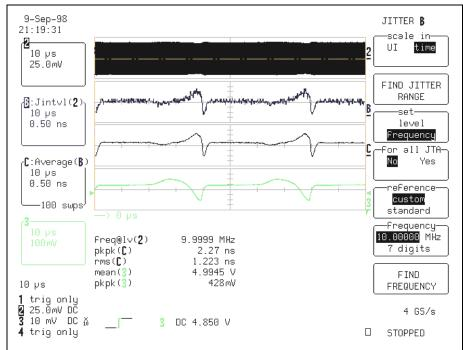
Figure 3 – Measuring effect of power supply ripple on an oscillator's output phase
