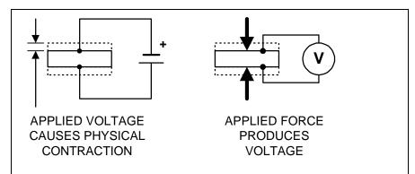
Figure 1 – Piezoelectricity converts a force applied to a crystal into an electric voltage and an applied voltage into a mechanical deformation
