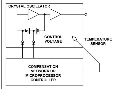
Figure 4 –Block diagram of a temperature controlled crystal oscillator (TCXO)
