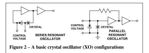
circuit it begins to oscillate at a frequency dependent primarily on the dimensions of the crystal. Figure 2 shows the basic crystal oscillator configurations.
